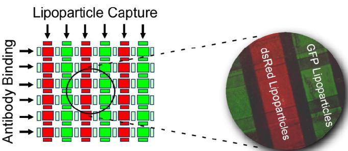
**Figure 1.** Schematic diagram of a ProteOn chip and fluorescence microscopy image of a GLC chip with immobilized Lipoparticles in verticle channels captured via the JS-81 antibody. Captured Lipoparticles contain either GFP or dsRed fluorescent proteins.
